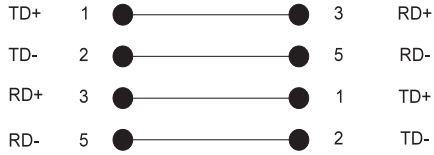
Figure A-3 10BASE-T Cabling
