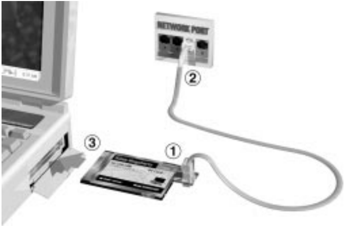
Figure 1-3 Connecting the CardBus PC Card
